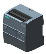
SIMATIC S7-1200, CPU 1212C, compact CPU, AC/DC/relay, onboard I/O: 8 DI 24 V DC; 6 DO relay 2 A; 2 AI 0-10 V DC, Power supply: AC 85-264 V AC at 47-63 Hz, Program/data memory 75 KB
